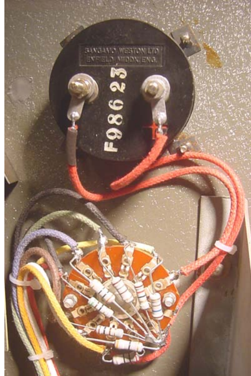
Above left: original meter shunts and switch (per Alan Ainslie's set), Above right, replacement meter shunt circuits in the SPARC museum set built using standard components. Below left: original detector/AGC/1 st audio stage module (beneath the shield per Alan Ainslie's set), Below right: replacement components in the SPARC museum set
