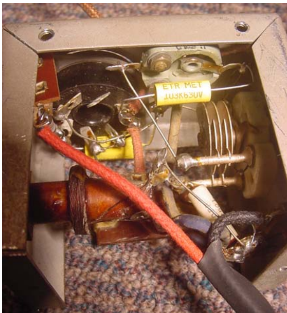
Above: BFO unit with new resistors and capacitors fitted. Note new flying leads
