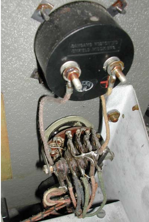
Above left: original meter shunts and switch (per Alan Ainslie's set), Above right, replacement meter shunt circuits in the SPARC museum set built using standard components. Below left: original detector/AGC/1 st audio stage module (beneath the shield per Alan Ainslie's set), Below right: replacement components in the SPARC museum set
